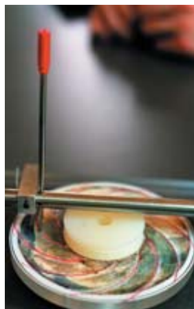
SCRATCH THAT: Replica of a machine possibly used to cut spirals on jade.
