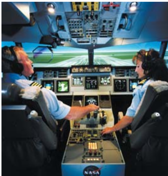
INTELLIGENT FLIGHT CONTROL has been tested in the mock cockpit (left) of the Advanced Concepts Flight Simulator (above) at the NASA Ames Research Center in California.
